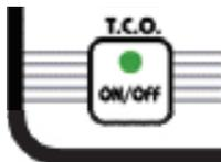
The optional “Time Clock Override” control you can set the switch turn this switch ON and the heater will start the water filter pump automatically whenever the water temperature drops below the thermostat setting.
