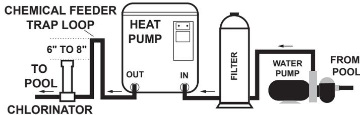
**2. CHOLORINATOR.** Be sure to install a **CHEMICAL TRAP LOOP** as shown. The loop should be at least 6 to 8 inches above the chlorinator/feeder top to prevent chlorine backup into the heater when the water pump is off. All feeders should be installed at the **same or below the heater piping elevation** to prevent chemical back up into the heater.
