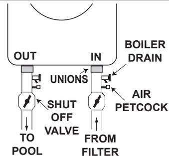
**4. BYPASS FOR FLOW RATES OVER 70 G.P.M.** Typically the automatic internal water bypass can handle up to a 1.5 H.P. water pump or 70 G.P.M. If the water pump exceeds 1.5 H.P. then install either of the optional bypasses as shown below. The installation of a flow meter on the WATER OUT line is suggested. Adjust the bypass to divert a minimum of 40 to 50 G.P. M. through the heater. Flow meters should be installed per the manufacturer's instructions.
