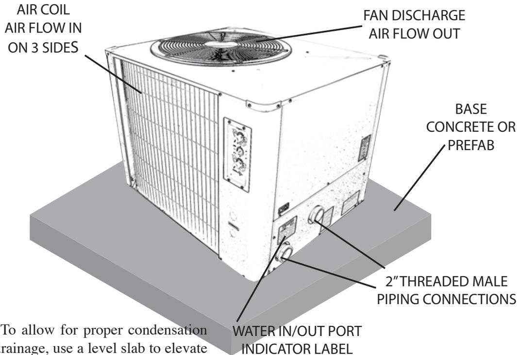
1. To allow for proper condensation drainage, use a level slab to elevate the heat pump to at least the same height as the pool filter system slab, or 2 to 3 inches minimum above grade.
